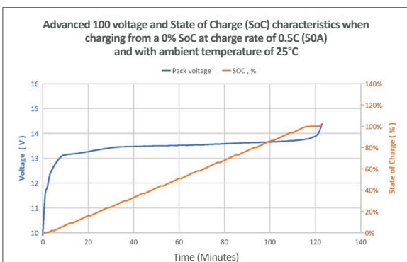
The C-rate is the charge or discharge rate that a battery is charged or discharged at.
